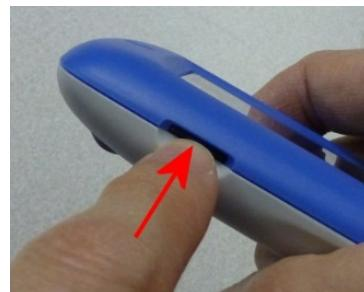
**Withdraw protruding memory card from slot**
